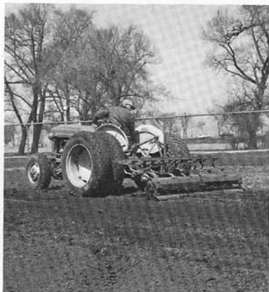
First, ground was thoroughly broken up and aerated by a Ford equipped with rotary tiller, above left. Then, above, ground was smoothed . . .
