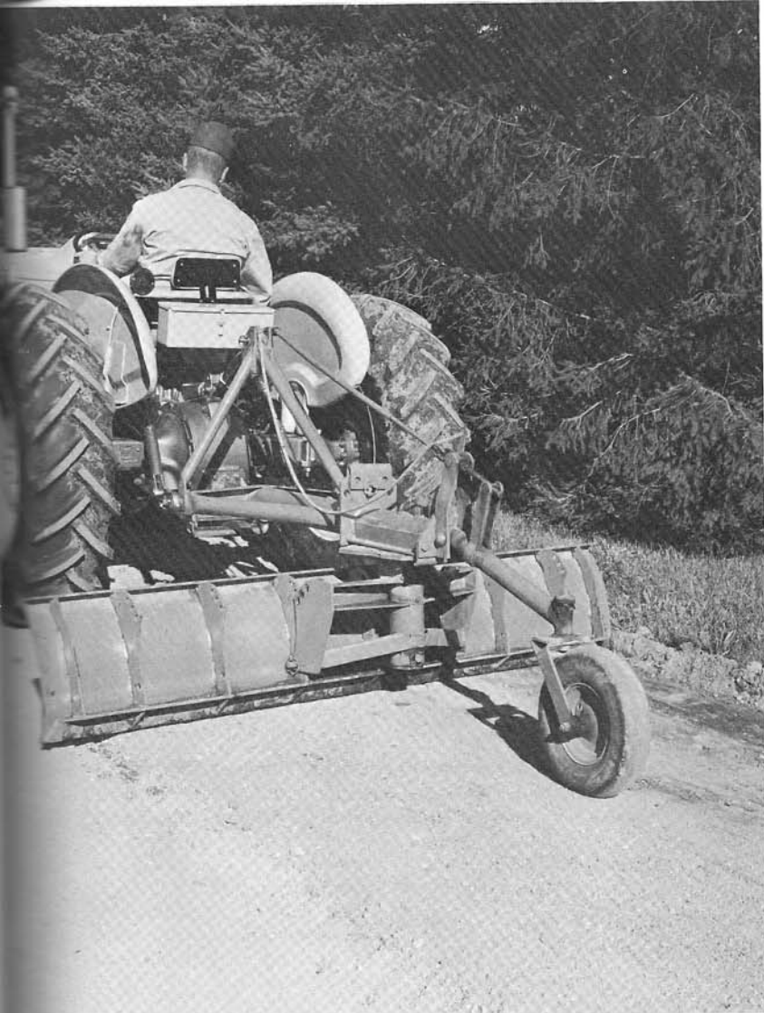
Ford 710 and 716 blades can be offset to work beyond the rear wheel tread, let operator work next to curbs, foundations, other obstacles.
