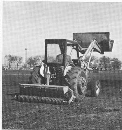
. . . by a Ford with landscape rake. Finally, area was quickly seeded by this Ford tractor equipped with a seeder-packer.
