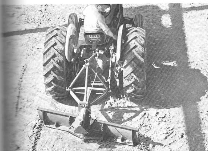
Ford blades can be readily angled to the right or left to windrow material either way. Ford 710 and 716 blades can be angled by the operator from his position on the tractor.
